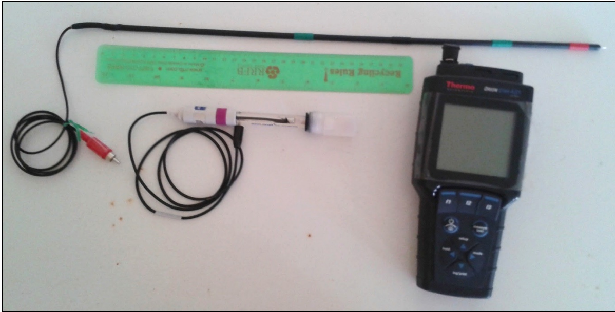
Figure 14 Constructed platinum electrodes (top), accumet calomel reference electrode (bottom) and Thermo Scientific Orion Star A221 Milivolt Meter. Photograph by C. Skinner 2013).
